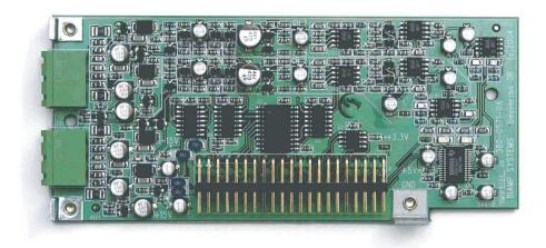
IP2 input cards allow each AudiaFLEX installation to have the quantity and type of inputs required. Each IP2 Card provides two channels of mic/line input, as part of AudiaFLEX hardware. Inputs are balanced, and are provided on plug-in barrier strip connectors. Software control of individual inputs includes: gain w/ peak indication; +48V phantom power; mute; level; and signal invert.
